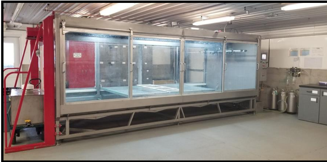
Figure 1: Multi nozzle spray chamber located at the PAT lab.
